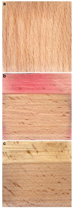
Fig. 3 Internal pigmentation by a dual inoculation, b pretreatment with sterilization and c pretreatment without sterilization
