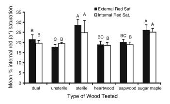
Fig. 1 External and internal red (a\*) saturation amounts on beech and sugar maple cubes. *Different letters* indicate significant differences at  $\alpha$ =0.05 for each surface. *N*=10
